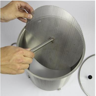
Once the bottom screen is in place use the extension tube and place this on top of the other stainless tube that you just attached to the bottom screen.
